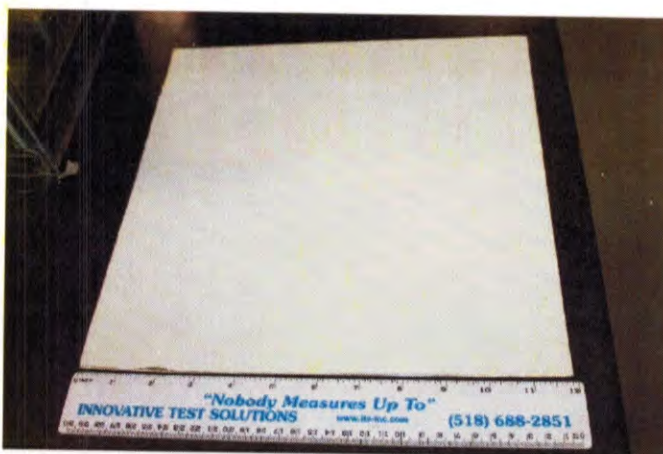
Figure 1: The Sectioned 1-foot X 1-foot test panel cut from the painted 36" X 48" panel.
