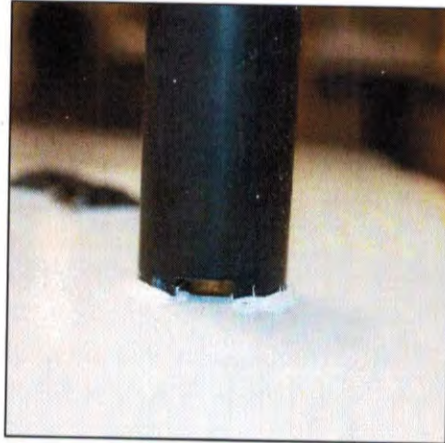
Figure 2: The plastic standoff adhered to the test panel.
